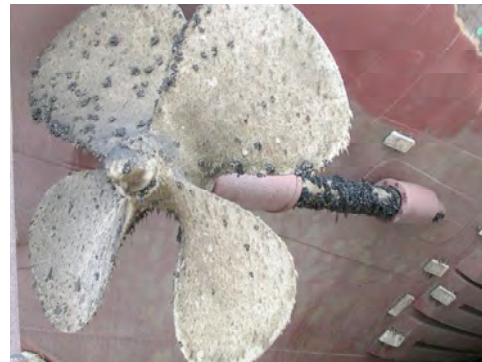
Fouling organisms, including bivalves and barnacles, on the propeller of a vessel examined in dry dock. Photo courtesy of California State Lands Commission
