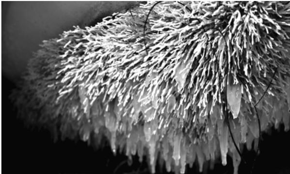
Twelve weeks' undisturbed fouling by invasive tubeworms (*Hydroides* sp.) and sea squirts/tunicates (*Ciona* sp.) on nontoxic, siloxane hull coating in San Diego Bay, October 20, 2005. Growth extends approximately 3 inches from hull surface.
