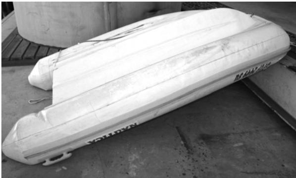
Hydro-washing easily removed tubeworms and sea squirts/tunicates from the same boat hull at a San Diego Bay boatyard, November 30, 2005.
