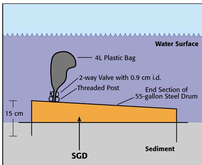
**Figure 3:** The seepage meter offers a simple, inexpensive method for measuring groundwater discharge into surface waters. This diagram shows the seepage meter placement in the sediments and its collection bag attachment. (Source: Florida Sea Grant)
