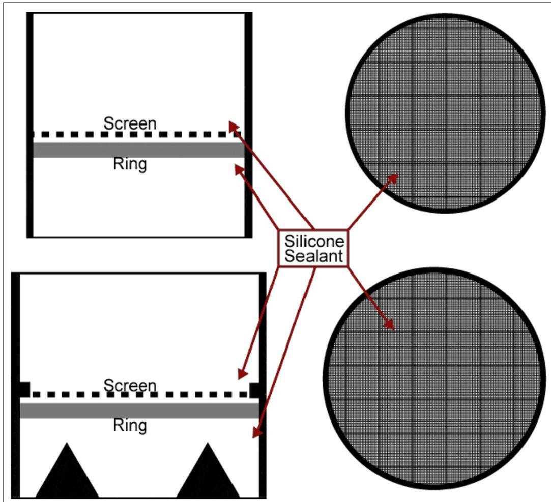
Figure 12. *Stacked sieves schematic.*
