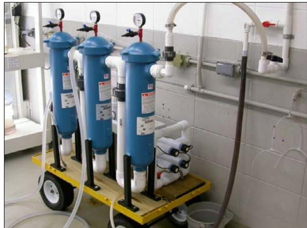
Figure 4. Filter set and ultraviolet sterilizer.
