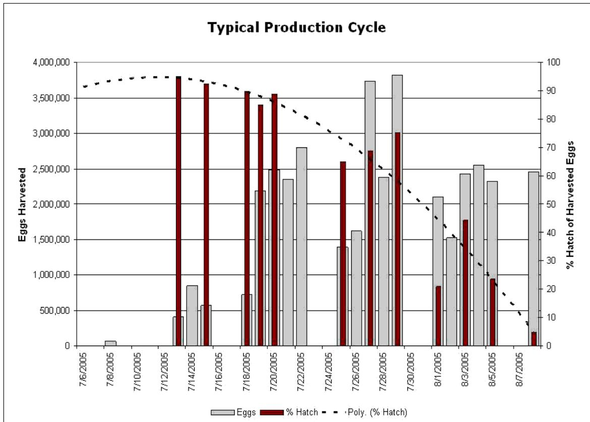
Figure 6. Typical Production Cycle. July 6 – August 8. Tank stocked with N3 – C1 A. tonsa at 1 per ml on July 6th. One week later egg production started. Two weeks later egg production began to peak. Three weeks later, egg production remained high, but the hatch % was declining. After four weeks of batch culture, hatch was below 25%.
