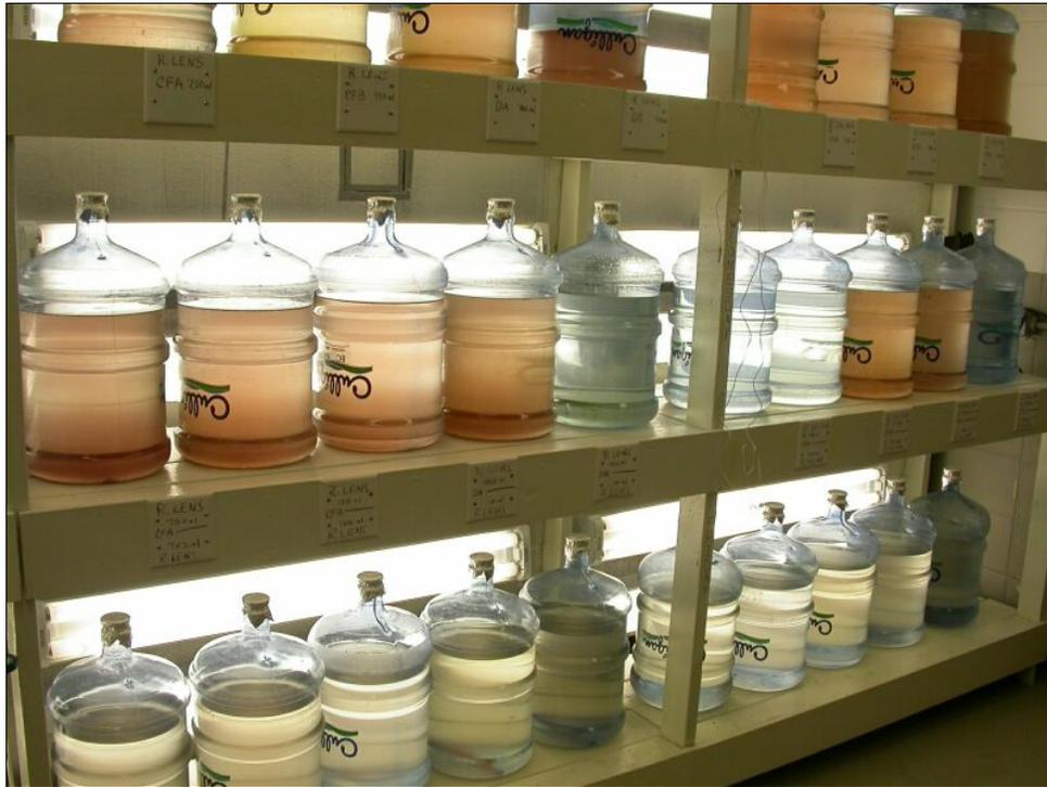
Figure 7. Carboy algae culture. Lights are maintained on an 18 h on / 6 h off cycle.
