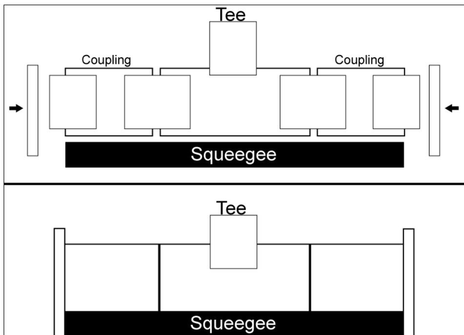
Figure 10. *Squeegee longitudinal section schematic.*
