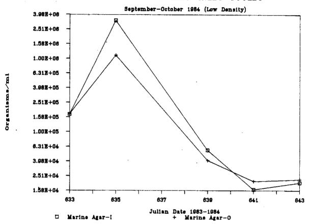
Figure 28. Mean inlet and outlet marine agar plate counts for the protein skimmer stocked at low densities (September-October, 1984)
