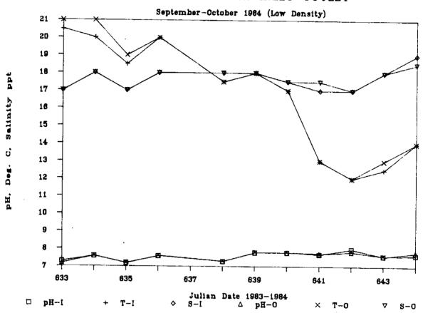
Figure 16. Inlet and outlet pH, temperature (°C), and salinity (ppt) levels for the protein skimmer stocked at low densities (September-October, 1984)
