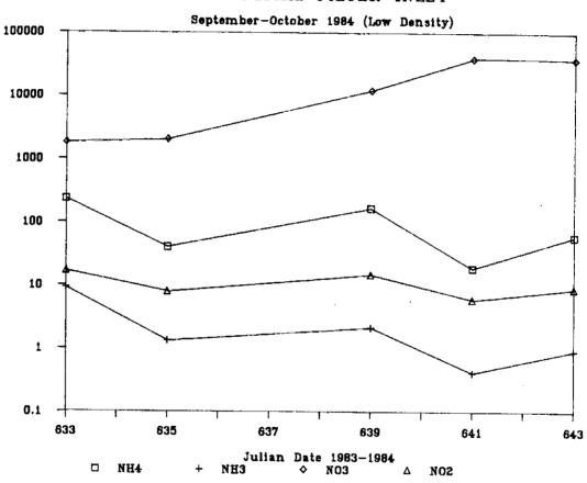
Figure 9. Mean inlet ammonium ( $NH_4$ ), ammonia ( $NH_3$ ), nitrate ( $NO_3$ ), and nitrite ( $NO_2$ ) levels for the biological filter stocked at low densities (September-October, 1984)
