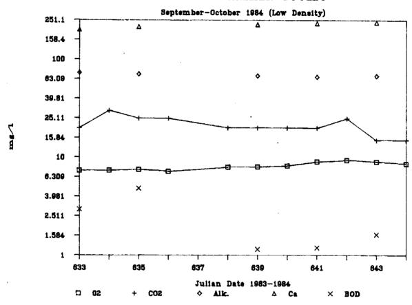
Figure 20. Mean outlet dissolved 02, dissolved C02, alkalinity, calcium, and BOD levels for the protein skimmer stocked at low densities (September-October, 1984)
