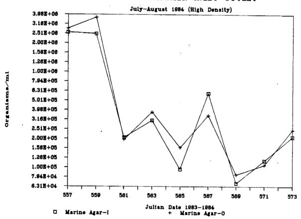
Figure 27. Mean inlet and outlet marine agar plate counts for the protein skimmer stocked at high densities (July-August, 1984)
