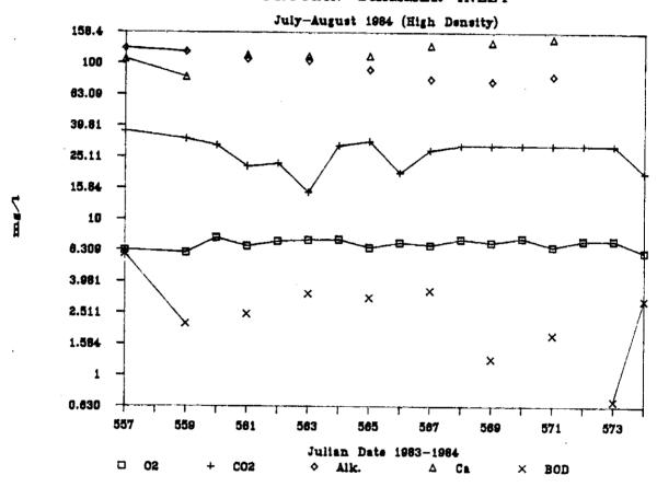
Figure 17. Mean inlet dissolved  $\rm O_2$ , dissolved  $\rm CO_2$ , alkalinity, calcium, and BOD levels for the protein skimmer stocked at high densities (July-August, 1984)
