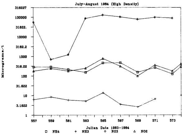
Figure 23. Mean inlet ammonium ( $NH_4$ ), ammonia ( $NH_3$ ), nitrate ( $NO_3$ ), and nitrite ( $NO_2$ ) levels for the protein skimmer stocked at high densities (July-August, 1984)
