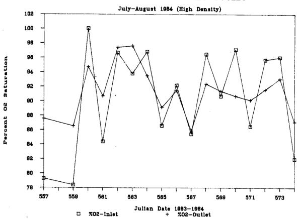
Figure 21. Mean inlet and outlet oxygen-saturation levels for the protein skimmer stocked at high densities (July-August, 1984)
