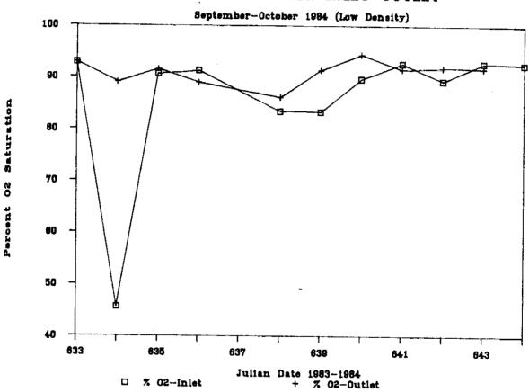
Figure 7. Mean inlet and outlet oxygen-saturation levels for the biological filter stocked at low densities (September-October, 1984)
