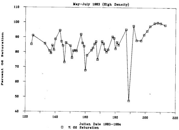
Figure 6. Mean outlet oxygen-saturation levels for the biological filter stocked at high densities (May-July, 1983)
