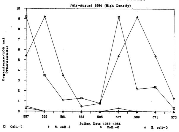
Figure 29. MPN total coliform and MPN  $\underline{E}$ . coli inlet and outlet populations for the protein skimmer stocked at high densities (July-August, 1984)
