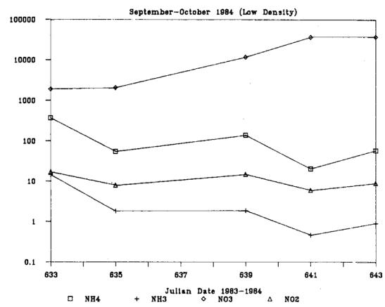
Figure 10. Mean outlet ammonium (NH $_4$ ), ammonia (NH $_3$ ), nitrate (NO $_3$ ), and nitrite (NO $_2$ ) levels for the biological filter stocked at low densities (September-October, 1984)
