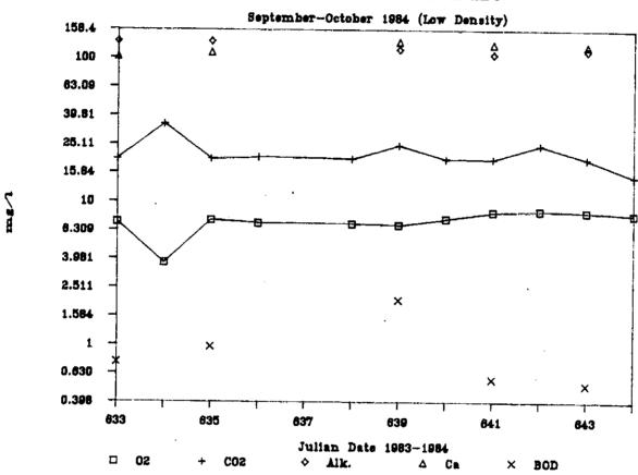
Figure 4. Mean inlet dissolved  $0_2$ , dissolved  $0_2$ , alkalinity, calcium, and BOD levels for the biological filter stocked at low densities (September-October, 1984)
