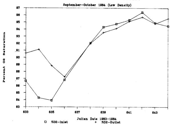
Figure 22. Mean inlet and outlet oxygen-saturation levels for the protein skimmer stocked at low densities (September-October, 1984)
