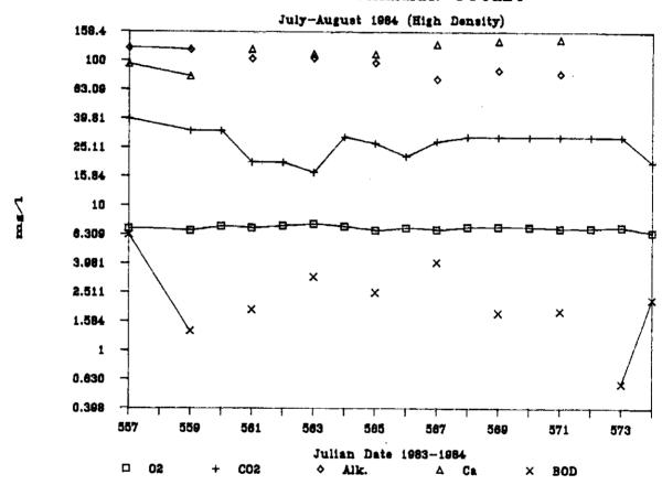
Figure 18. Mean outlet dissolved 0<sub>2</sub>, dissolved CO<sub>2</sub>, alkalinity, calcium, and BOD levels for the protein skimmer stocked at high densities (July-August, 1984)
