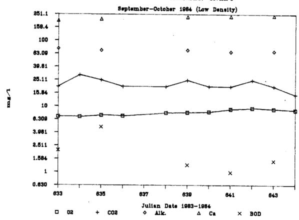
Figure 19. Mean inlet dissolved  $O_2$ , dissolved  $CO_2$ , alkalinity, calcium, and BOD levels for the protein skimmer stocked at low densities (September-October, 1984)
