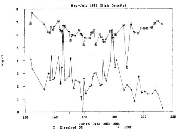
Figure 3. Outlet dissolved oxygen and BOD levels for the biological filter stocked at high densities (May-July, 1983)
