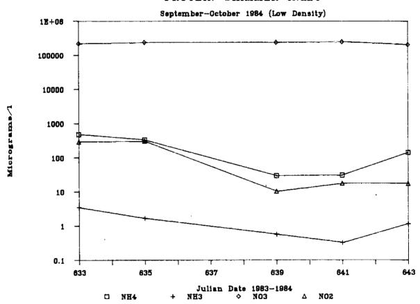
Figure 25. Mean inlet ammonium (NH $_4$ ), ammonia (NH $_3$ ), nitrate (NO $_3$ ), and nitrite (NO $_2$ ) levels for the protein skimmer stocked at low densities (September-October, 1984)
