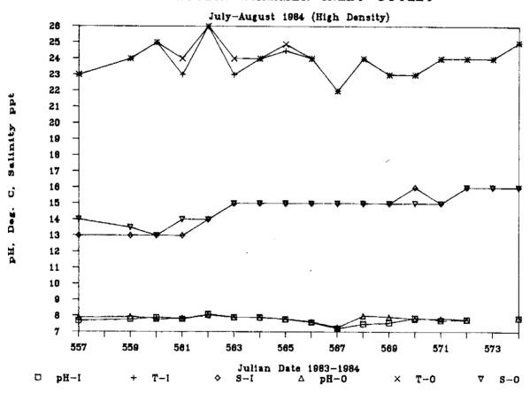
Figure 15. Inlet and outlet pH, temperature (°C), and salinity (ppt) levels for the protein skimmer stocked at high densities (July-August, 1984)
