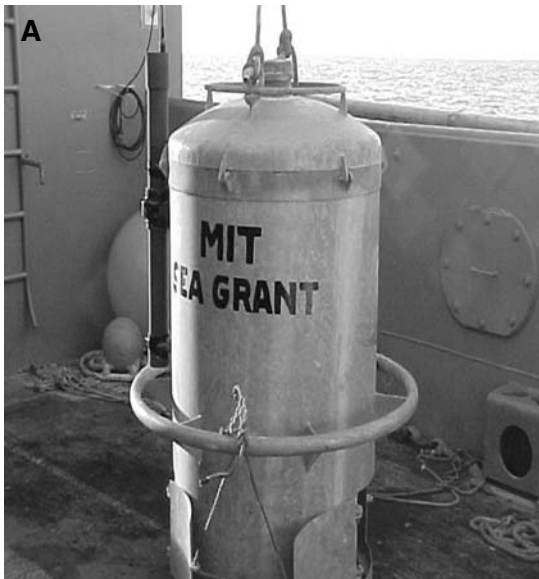
Fig. 5. The MIT Robofeeder (A) is attached to the top of the cage for autonomous fish feeding with feed placed in the silo and falling through two hoses exiting the spar (B).
