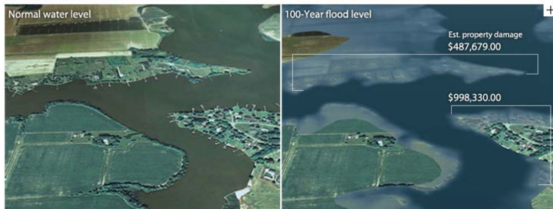
(left) Homes and docks along Fishing Creek, on Maryland's Eastern Shore, at normal water level. (right) Water level during a once-in-a-century flood and an estimate of resulting property damage. (Images by Hunter Allen and Richard Rivera, based on Digital Flood Insurance Rate Maps and imagery provided by Michael Scott, Salisbury University.)
