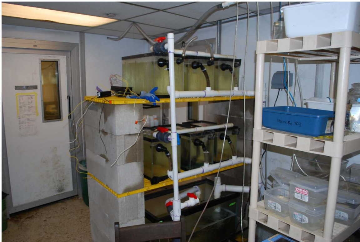
Figure 6: Experimental setup #1 Cunner and Green Urchins in the top aquariums, Ulva lactuca in the middle aquariums, and a mixing reservoir in the bottom. Setup #2 is identical other than the absence of Tautoglabrus adspersus in the top aquariums.
