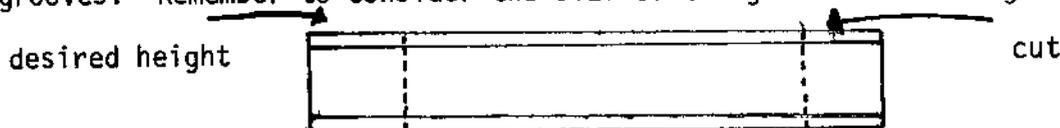
Once the ends have been cut, the glass should be placed on the base and centered. With the glass in the grooves, place the ends on the glass. There should be enough room left on the base to allow for the addition of the end brace. Mark the position of the end pieces then remove the ends and glass.
