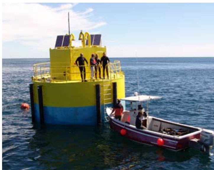
A 20-ton, floating container for supplying feed to offshore caged fish.
