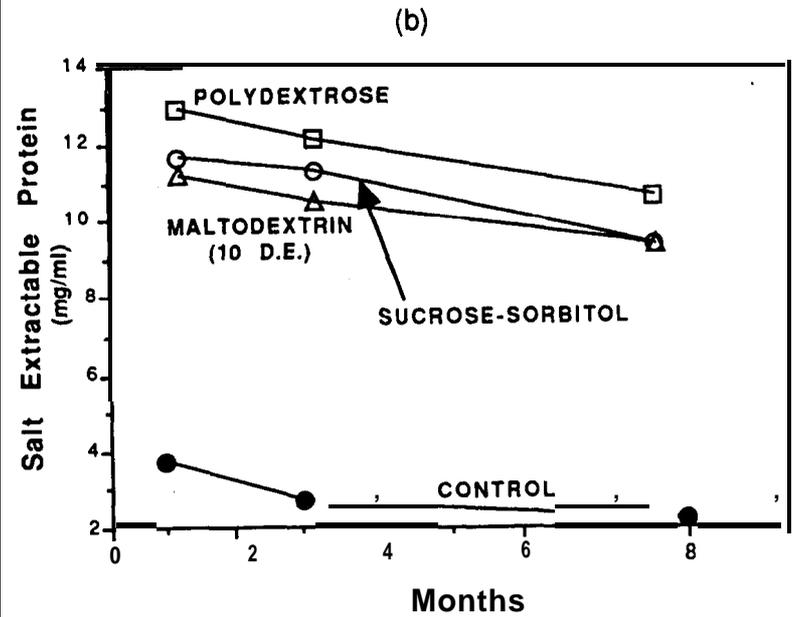
Figure 2: Surimi: Effects of added cytoplasmic components on maintenance of (a) gel-firming properties and (b) protein extractability during frozen storage. Stress and strain at failure correspond to the strength and cohesiveness, respectively, of heat set gels prepared from surimi containing 2% salt.
