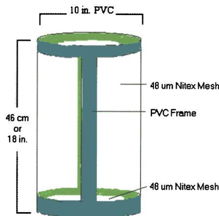
Fig. 5. Rearing chamber
