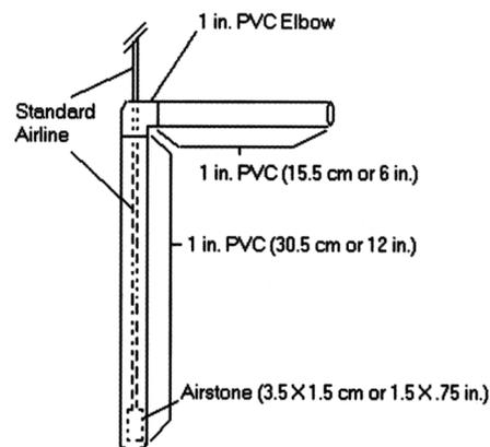
Fig. 6. Stand pipe used in the hatching and rearing chamber
