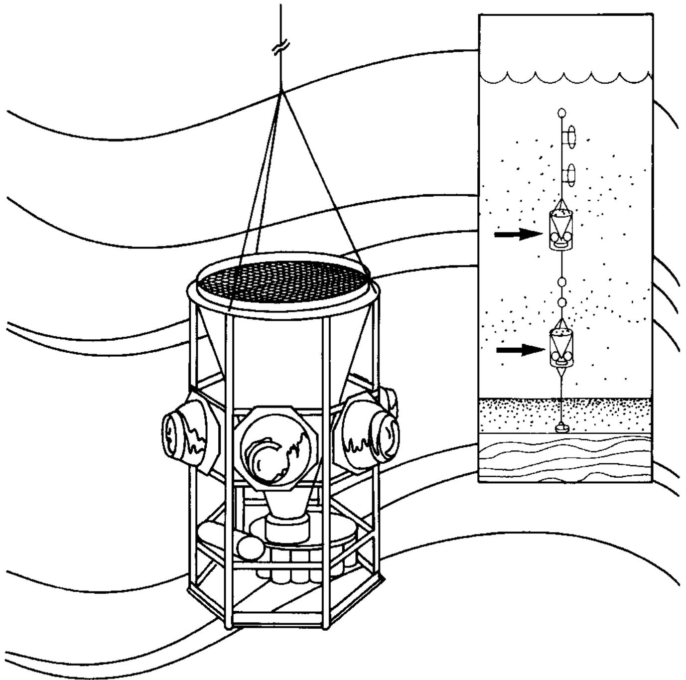
Studying the sediments found on different parts of the ocean floor helps marine geologists understand more about the past and present of the area. They use **sediment traps** to collect particles settling from the surface of the ocean to the seafloor. Many of the sediments, like mud, sand, or clay come from land and were carried to the ocean by rivers, streams, or winds; some started out in other parts of the ocean but were moved around by currents or waves.
