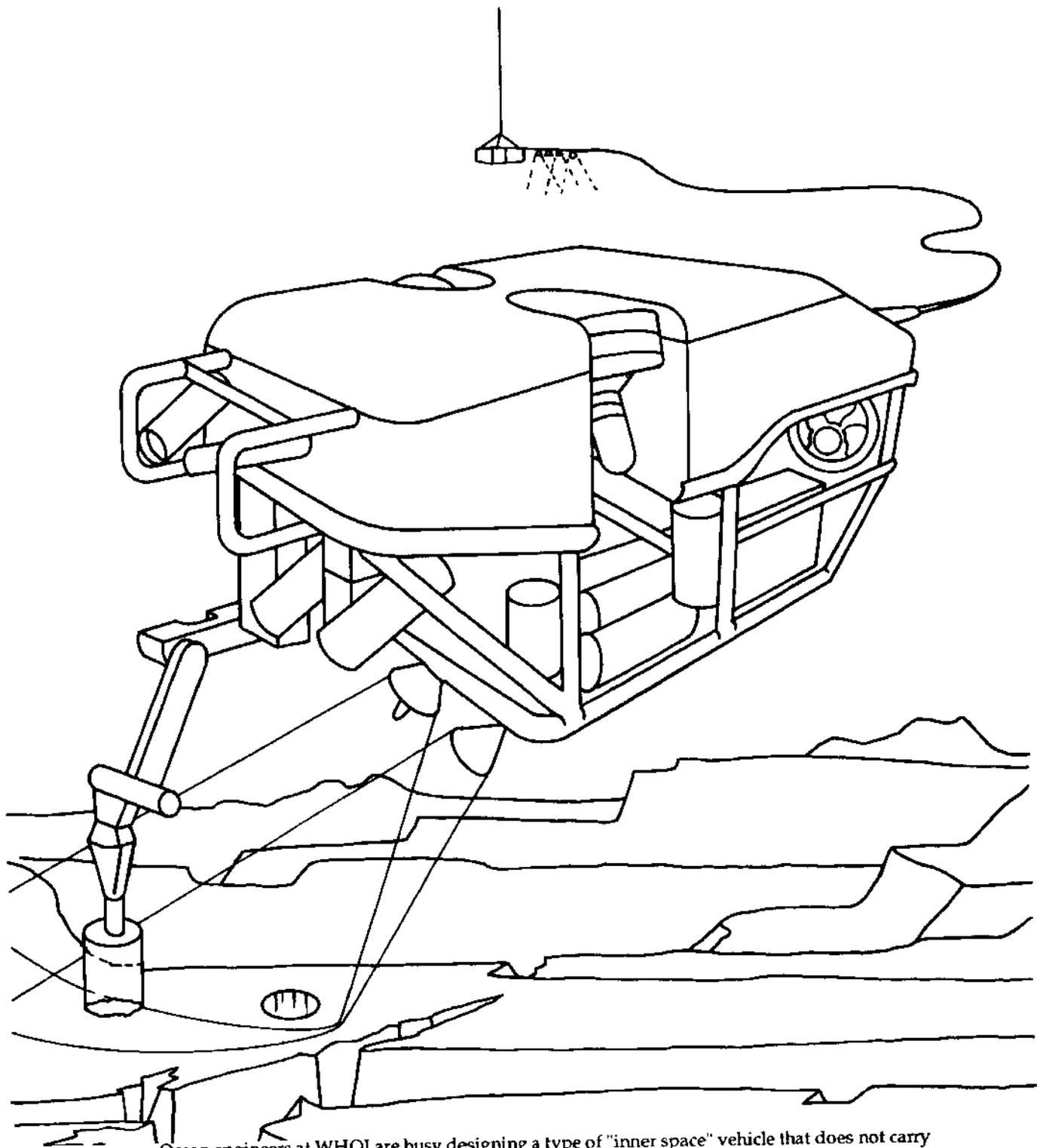
Ocean engineers at WHOI are busy designing a type of "inner space" vehicle that does not carry people. They can go deeper into the ocean and stay down longer than manned vehicles. Called **remotely operated vehicles**, or ROVs, these robots are remotely controlled by a researcher seated comfortably aboard a ship. Lights and cameras mounted on the ROV illuminate the underwater world and send pictures to the surface through special cables that connect the ROV to the ship above.
