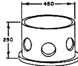
Figure 4: Modular structures, usually of concrete, are in greater use in the world's artificial reefs.
