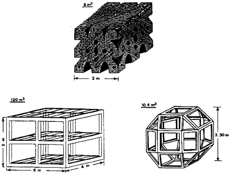
**Figure 3: Examples of artificial reefs fabricated according to highly controlled aspects of composition and construction. (facing page, structures from Japan; this page, Mediterranean Sea.)**
