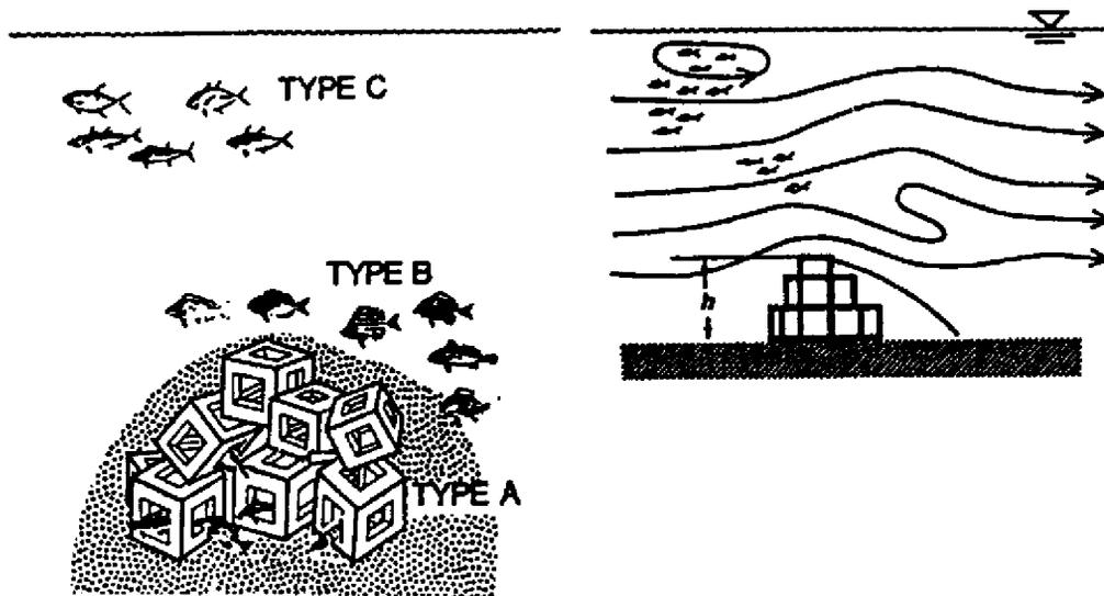
**Figure 5: Japanese research has characterized the affinity of some fishes to artificial reefs as (A) benthic dwellers in physical contact with it, (B) linked to it visually only, and (C) at some distance to it. The latter group might be in a "lee wave." (Redrawn from Grove *et al.*, 1991)**
