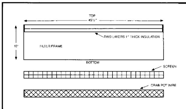
**Figure 2: the freshwater filter**
