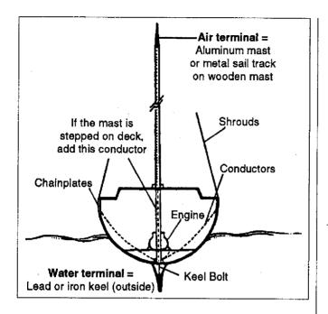
A complete lightning protection system has four components:
