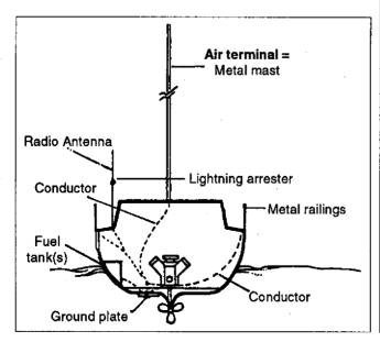
Do not use a radio antenna as an air terminal or attempt to take an antenna down during a thunderstorm. Instead equip all antennas with a lightning arrester in the lead-in cable. The iiahtnina arrester allows normal operation of the radio, but in the event of a lightning strike to the antenna, the high voltage iumps a small gap within the arrester and is shunted to ground. It not only provides protection for the vessel, but reduces the chance of damage to the radio equipment.
